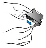
8 Push the black print cartridge firmly down into the slot on the right.
